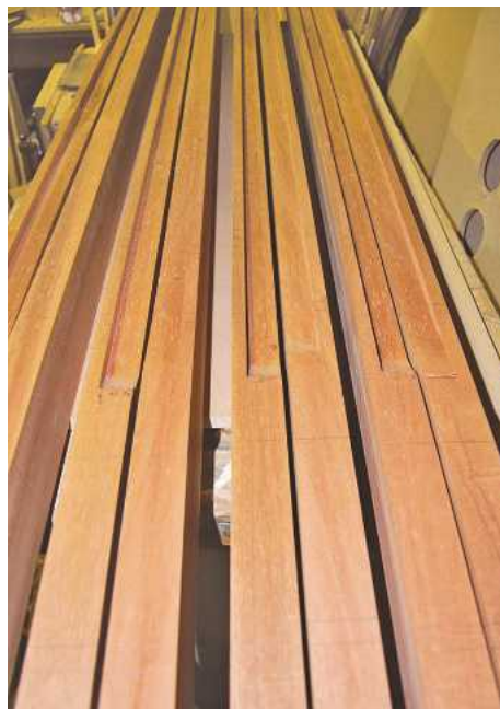
▲ Pic.7 The rebated stiles, completed and ready to be fitted
